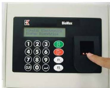
Terminal BioMax FP: plastic case
